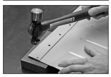
4 Strike the back of each rivet with a hammer until flattened TIGHTLY against the back of the new wear strip. (Soft smash-down rivets are provided so no special tool is needed.)
