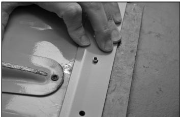
3 Lay the shovel face down on a hard surface such as an anvil or solid concrete. Place the new wear strip along the BACK of the blade. Working with one rivet at a time, push rivets from the FRONT through holes in blade then wear strip.
